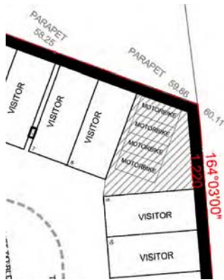
Figure 2.3: Insufficient Access to Motorcycle Parking Spaces
